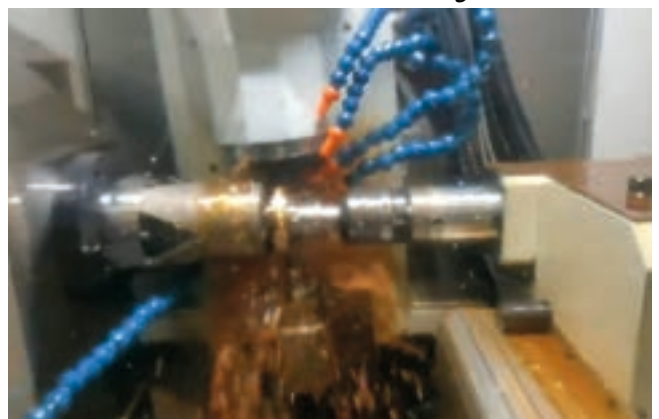
Dentatura corona - Worm wheel toothing
