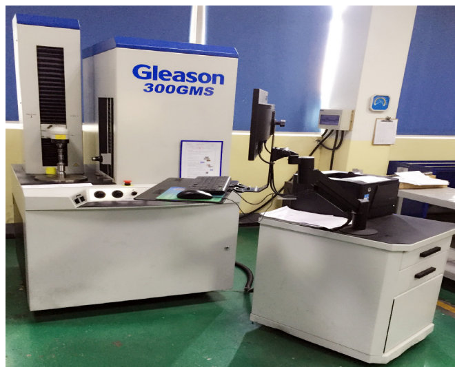
Evolventimetro - Involute pitch gauge
