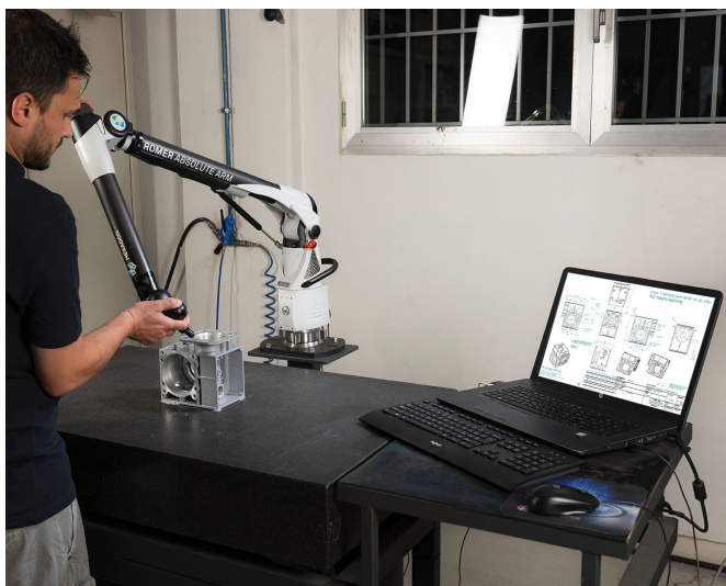
Braccio meccanico - Three-dimensional mechanical arm
