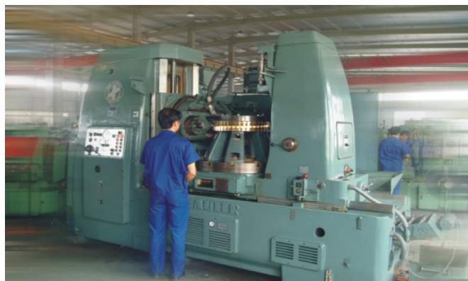
Dentatura corona - Worm wheel tooth grinding
